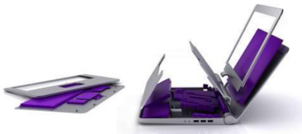
Figure 1. Bloom Laptop Modular Design (Bohbe et al 2010)
