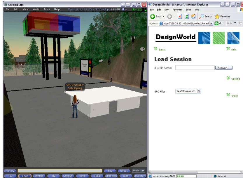
Figure 5. A simple house model uploaded from a .ifc file.
