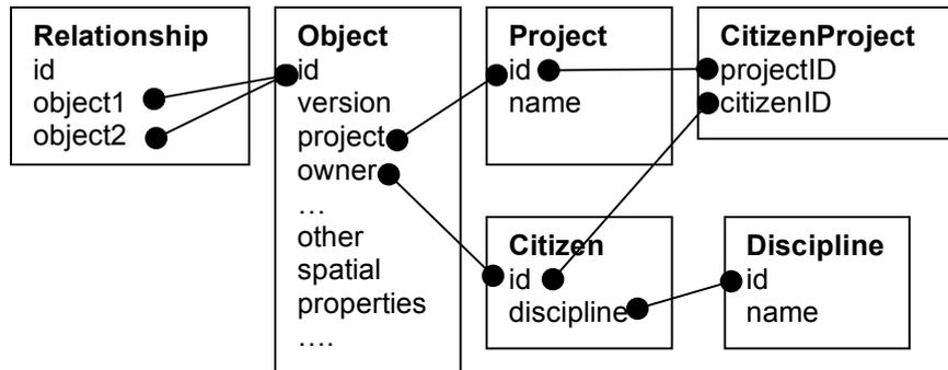
Figure 3. Overview of the DesignWorld external model schema.
